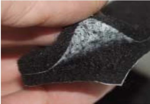
MagicFleece is a two-layered sound absorbing fleece. It is composed of countless polyester microfibrers that are woven into a smooth compound using advanced fibre processing technology. The open structure of MagicFleece lets the noise penetrate deeply into the material, where it is absorbed efficiently due to the enormous surface area inside the fleece.
