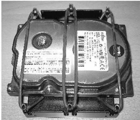
This is what the completed assembly should look like. Adjust the rubber tension so that the disk does not quite touch the rubber buffers. This is accomplished by tugging the rubber bands slightly around the four corner hooks, thereby redistributing the tension between the upper and lower parts of the rubber bands.
